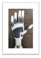
The ADL arm is entirely 3D printed and through a variety of tests conducted using the Anthropomorphic Hand Assessment Protocol as well as the usability assessment, the ADL arm was found to be functionally competent, relatively acceptable with proven ability to assist in the performance of ADLs in a simulated-use environment.
