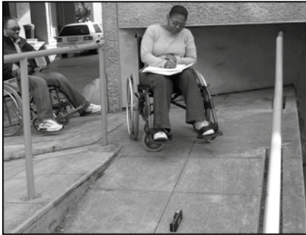
(a) Ramp gradient measurement 5
