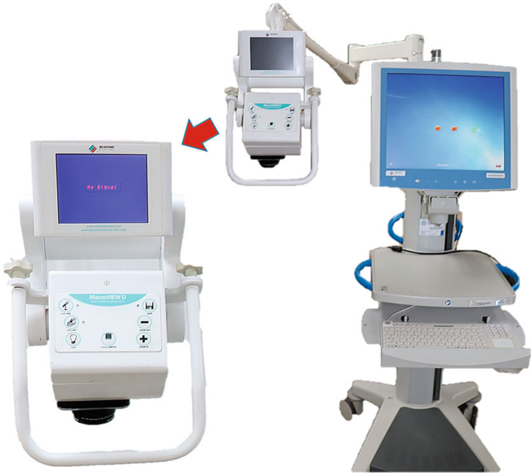
Fig. 8.6 Mobile MacroView DM 5 imaging unit with high definition (HD) camera fitted on spring, height adjustable arm with the control panel on the digital imaging module
