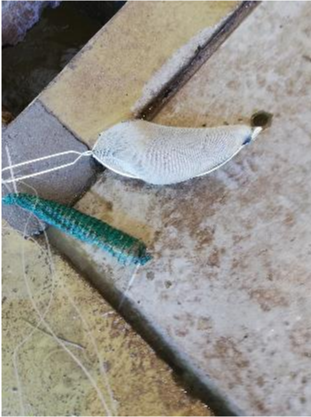
Passive samplers inserted as the waste is being emptied into WWTW by tanker
