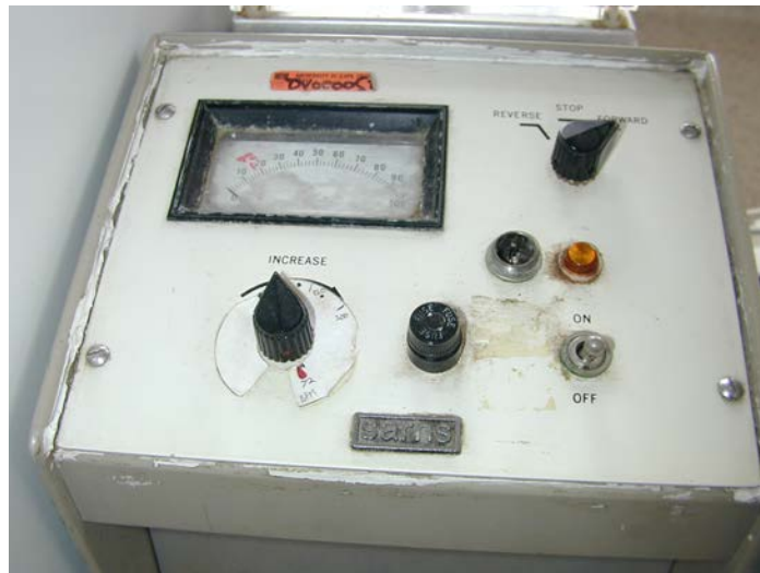
Figure 2-7: The controller for the roller pump
