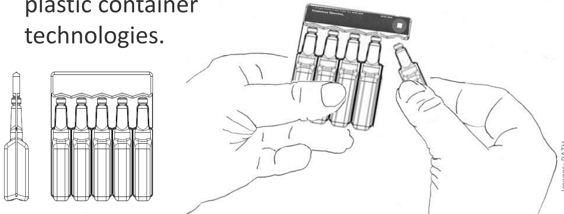
CAD models of multi-mono-dose design.
