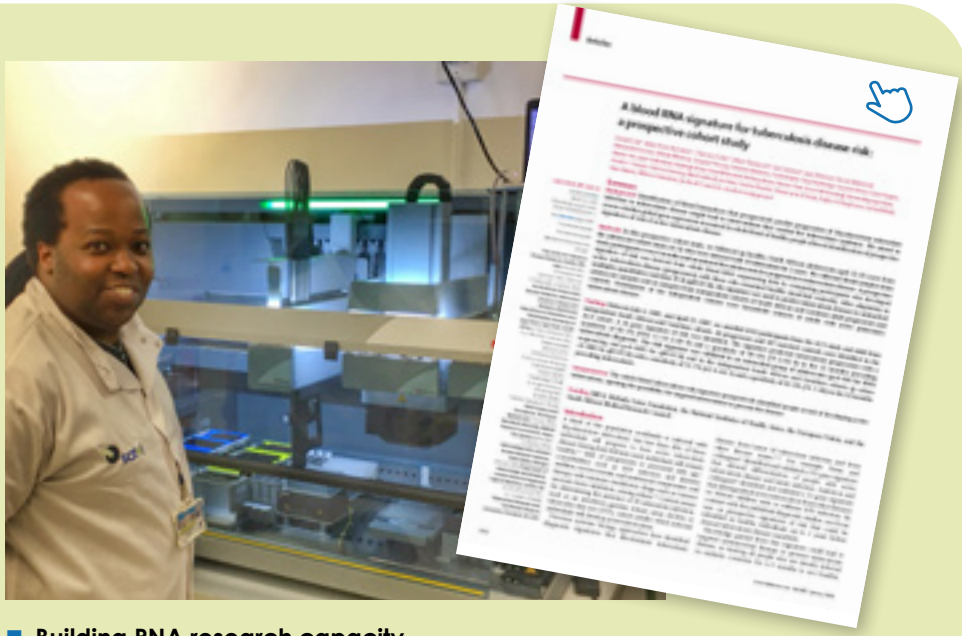
■ Building RNA research capacity During June 2016 SATVI acquired a Tecan Freedom EVO 150, a core liquid handling and robotics workstation to increase the capacity for high-volume RNA extraction from blood samples. This equipment allowed screening of more than 20,000 individuals for possible inclusion in the CORTIS-01 trial. Depicted is Senior Technologist Mzwandile Erasmus with the Tecan Freedom EVO workstation.
