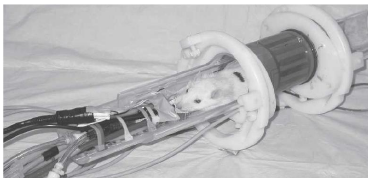
Figure 2.14: A 250 g rat prepared for imaging in a 2T system using a 6 cm diameter birdcage coil. The animal is lying on a Plexiglas cradle and is anesthetized with isoflurane delivered by mechanical ventilation. The hoses to the left are for ventilation gases and the black cables carry signals from ECG electrodes on the foot pads, airway pressure transducer on the breathing valve attached to the
