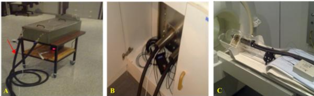
Figure 3.17: Set up at CUBIC before initiation of rat imaging. A) Water tank connected to the cradle via insulated tubing (arrow). B) Insulated tubing passing through the waveguide. C) Cradle positioned in the RF coil on the MRI bed.
