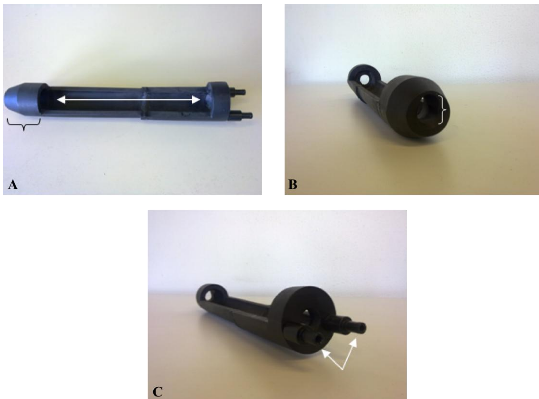
Figure 3.5: Images of the cradle at different views. A) Top view shows rat's resting area (arrow) and nose cone (curly bracket). B) Front view showing inlet for anesthetics (curly bracket). C) Inlet and outlet of hot water (arrows).
