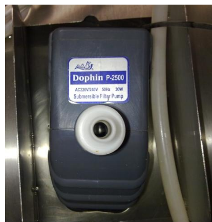
Figure 3.15: Water pump (Dolphin P-2500) used for transferring water from the tank to the cradle, and vice versa.
