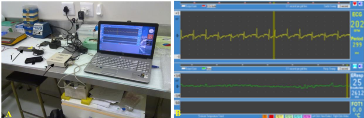
Figure 3.13: Images of modules and a notebook displaying ECG signals. A) ECG/Temperature module (arrow 1) transferring data to Control module (arrow 2), which is responsible for transmitting data to the notebook. B) ECG signals displayed using software, called PC-SAM. No respiration signals are observed on the software as they are magnetic field dependent.
